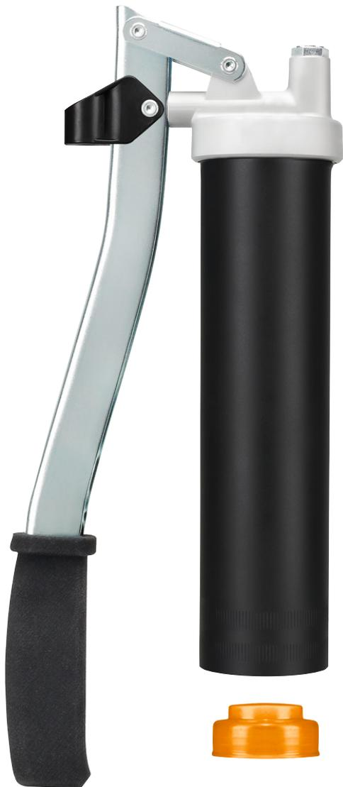
The new easyFILL 400 works without the need of any spring mechanism. Simply insert the cartridge, insert the follower plate and get started. The vacuum in the grease gun head moves the piston smoothly upwards all by itself. Through the Variable Stroke principle the grease gun can be easily operated with minimal lever movement.
