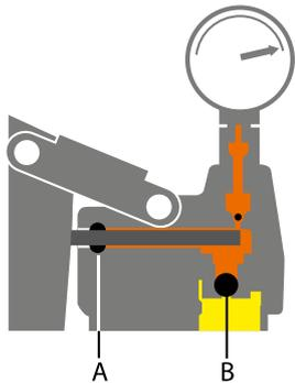
The check valve ensures lubrication even when using cold or viscous grease.
