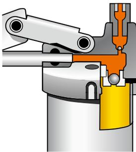
Lever position to obtain maximum delivery (approx. 1,4 cm<sup>3</sup> per stroke).
