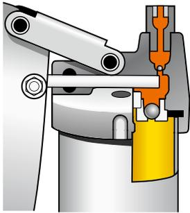
Hand lever position to overcome strong back-pressure, e.g. due to gummy lubrication point.
